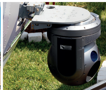
The multi-mission Kodiak 900 is towed to Daher Aircraft's EAA AirVenture exhibit stand after arriving at Oshkosh's Wittman Regional Airport (photo, left). A close-up (at right) shows the sensor turret after deployment through sliding sections in the aircraft's modified lower cargo door.
