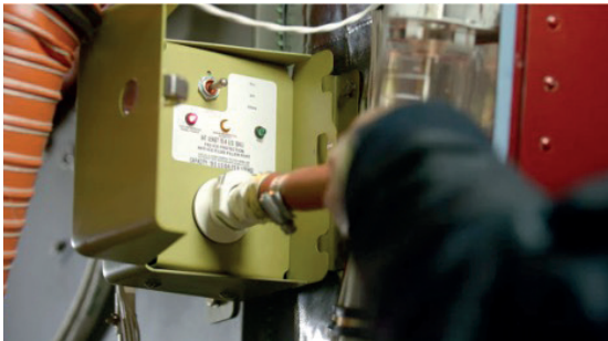
The Kodiak 900's automatic filling system for TKS anti-icing fluid is controlled by a panel in the engine compartment.
