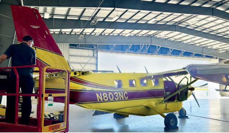
The Kodiak 100 operated by North Carolina Forest Service's Aviation Division undergoes the replacement of its elevators and repair of the rudder by Daher's TBM & Kodiak Care team at Asheville Regional Airport.
